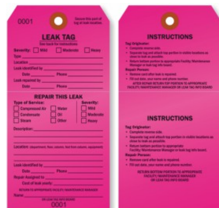
Figure 47: Red tag System for Compressed air leakage Reduction
